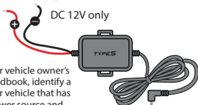
Refer to your vehicle owner's manual/handbook, identify a place in your vehicle that has constant power source and connect the DC 12V hardwire cable to it. Hardwiring by qualified professionals only.
